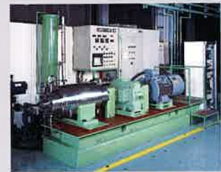
DRY GAS SEAL TEST BENCH
