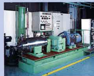
DRY GAS SEAL TEST BENCH
